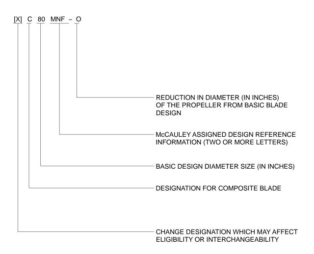
Propeller Model Designation Figure 4 (Sheet 2)
