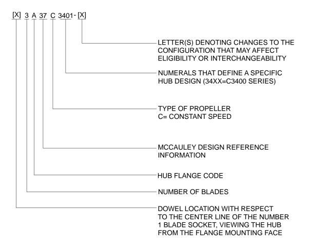
**NOTE:** A SPECIFIC PROPELLER ASSEMBLY IS IDENTIFIED BY THE HUB SERIAL NUMBER WHICH IS STAMPED ON THE HUB. ALL RECORDS OF PROPELLER COMPONENTS ARE KEPT WITH REFERENCE TO HUB SERIAL NUMBER. THE FIRST TWO DIGITS OF THE HUB SERIAL ARE THE YEAR OF MANUFACTURE. THE REMAINING DIGITS ARE THE NUMBER OF THE HUB MANUFACTURED IN THAT YEAR.
