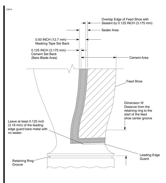
Propeller Anti-ice Feed Shoes Figure 201 (Sheet 2) 2614T1082
