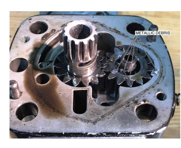
Figure 1. Metallic Debris Example (Sheet 1)
